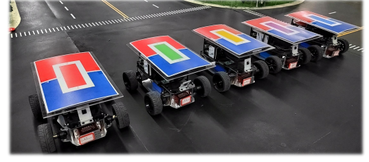
Fig. 4. Experimental robotic mini-vehicles. The mini-vehicles receive velocity and steering angles commands from the cloud server, and have on-board actuators (motors and steering gears) to execute these commands. A piece of colored cardboard is stuck to the top of each vehicle for vehicle localization via cameras installed on the ceiling.
